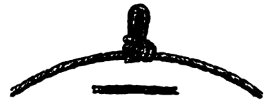
FIG. 2.—The Hornsby Knot as tied by the String-binder.
